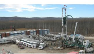
High Rate Annular Coiled Tubing Fracturing Operation (2015,
